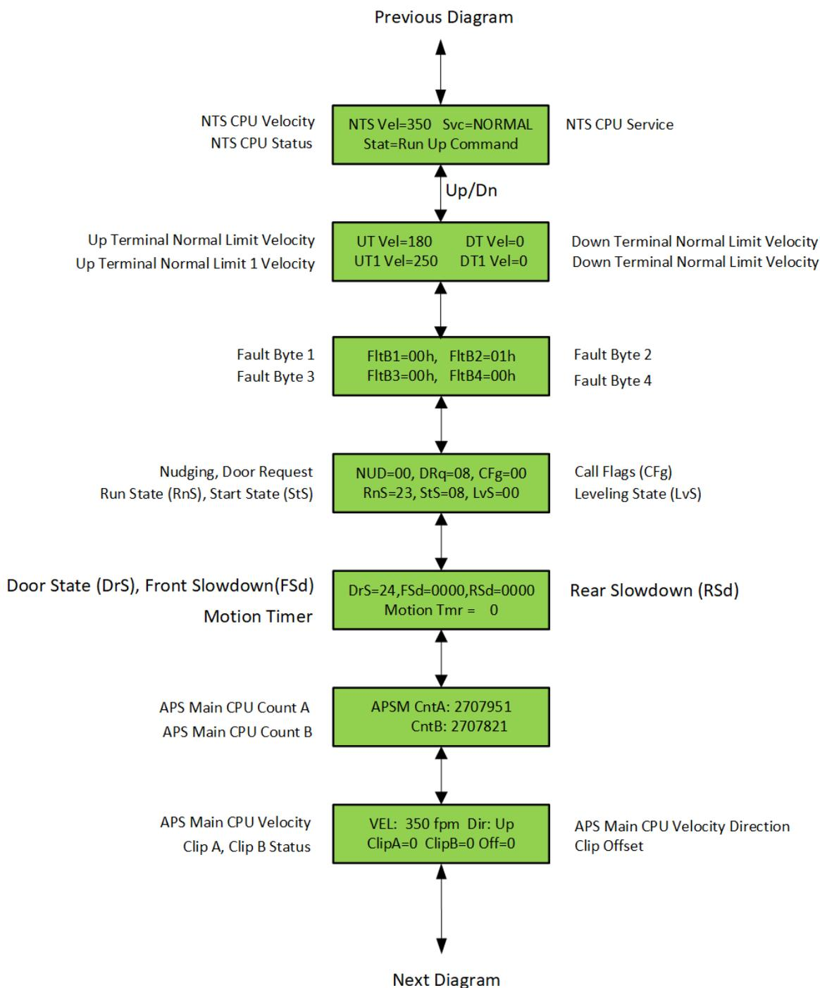
**Figure 5-2 B: LCD Interface Main Menu – Elevator Status**
